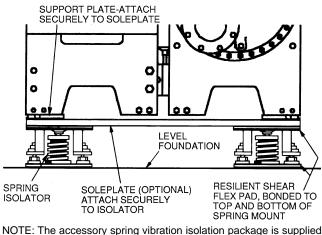
NOTE: The accessory spring vibration isolation package is supplied by Carrier for installation in the field.
